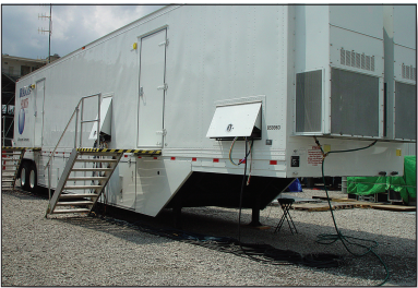
Figure 2.146 Another trailer often found at racing venue. This trailer is owned by Broadcast Sports, who facilitates a lot of the RF or wireless technology used for racing. This truck contains the RF receive and the two-way telemetry equipment for the in-car cameras that show viewers the track from the driver's vantage point. The signals from up to eight cars are radiated up to a helicopter, which retransmits them to this truck.
