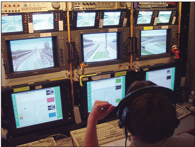
Figure 2.145 Inside the virtual graphics truck. The football field on the center monitor and the sign on the extreme left portion of the screen on the right monitor are computer-generated.
