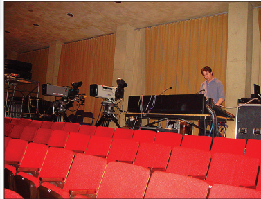
Figure 2.140 Many shows will require a PA system for the live audience. A separate vendor is usually called in for that effort, and usually sets their audio board where they can see the action.
