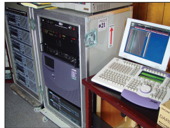
Figure 2.139 In the left case are six, eight-channel digital audio tape (DAT) recorders, which allow up to 48 channels of audio to be recorded for backup. The main recording device is the blue box in the right case. It is a specialized computer server that has software that makes it an audio workstation. Audio recorded directly by this workstation can be mixed and processed within the box. On the monitor to the right is the GUI for controlling the workstation.
