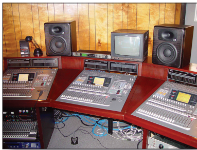
Figure 2.138 If the show is a music show, a separate audio recording company will often be brought in to record the audio as a mix and also as separate tracks for processing (sweetening) later or to produce tracks that will be released. The mix of the band is often done in a separate truck, or as the case here, in an adjoining office trailer. Then it is handed off to the television production truck's audio mixer for inclusion in the televised show. The audio recording vendor usually has two or possibly more technicians on site, depending on the complexities of the shoot. They usually set up at the same time as the production truck.
