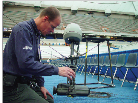
Figure 2.137 This is a skycam under inspection by a technician. The four cables connected to the center shaft work in concert to allow the camera to "fly" around and above the action. A crew of four supports this system and, again, can arrive up to a week before the event to install the system.
