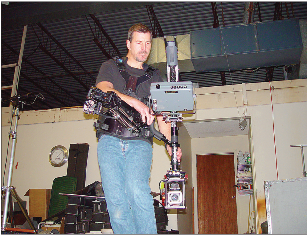
Figure 2.135 Steadicam operator. This harness and arm-to-camera pole allows for smooth and interesting camera moves. The pole the camera is on can be oriented for the camera to give a low perspective, as is the case here, or the setup can be inverted to get an over-the-shoulder look. Many operators own their own gear, so you are hiring them and their gear. There is a school conducted by the manufacturer for operators to hone their skills.
