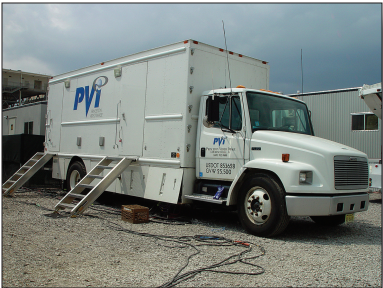
Figure 2.146 Another trailer often found at racing venue. This trailer is owned by Broadcast Sports, who facilitates a lot of the RF or wireless technology used for racing. This truck contains the RF receive and the two-way telemetry equipment for the in-car cameras that show viewers the track from the driver's vantage point. The signals from up to eight cars are radiated up to a helicopter, which retransmits them to this truck.
