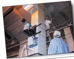
Figure 2.136 One of the cameras used in Eyevision, a unique system that uses multiple cameras to record the action in unison, so that upon playback the viewer's perspective can be changed as the play is reviewed. A crew of three or four, and up to a week, can be required for installation and setup. (Source: Core Digital Technologies/SWTv)
